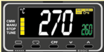
Example of an over-temperature limiter
