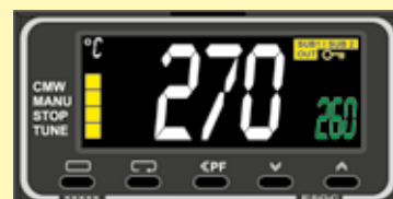
Example of an over-temperature limiter
